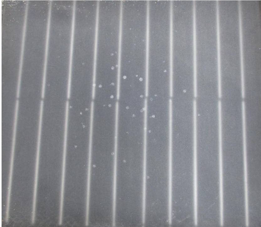
Figure 2 Surface damage caused by the sphere drop, before reaching the breaking height
