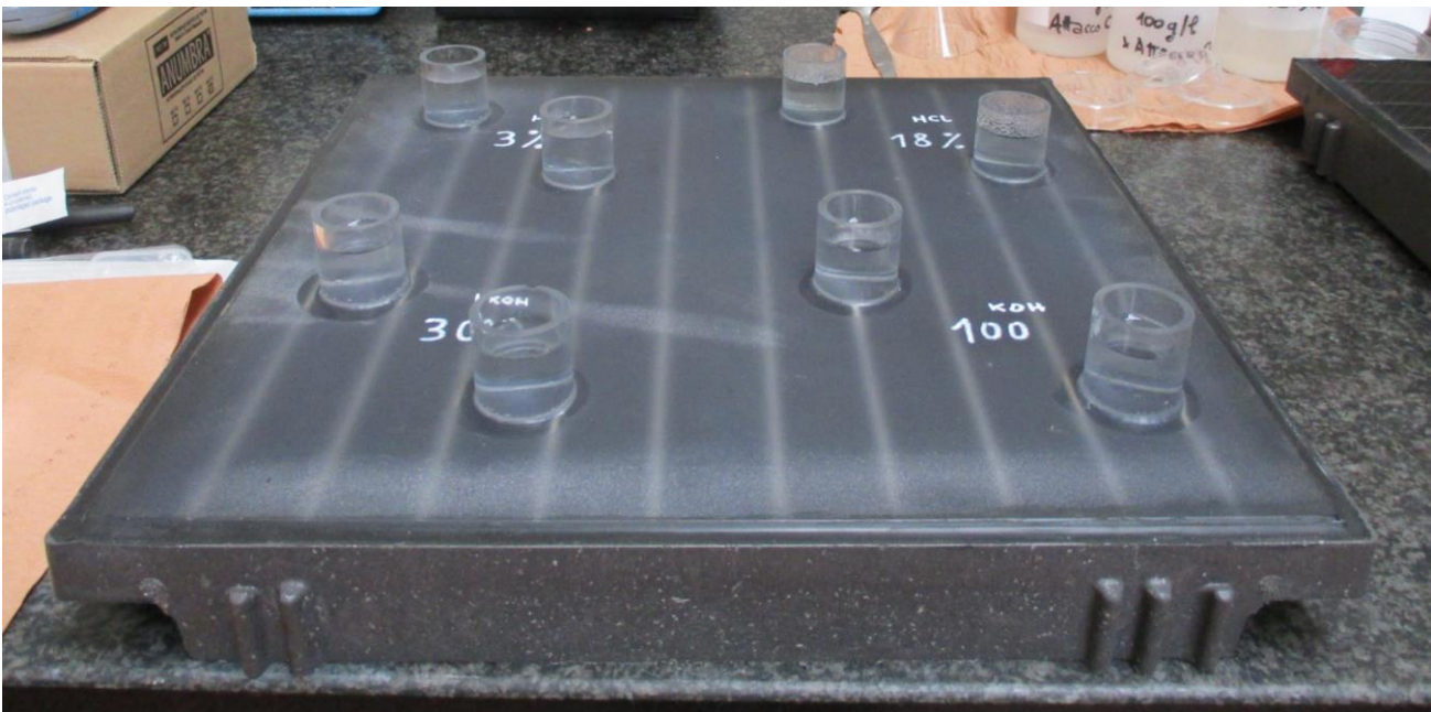
Figure 2 Surface of a sample in contact with the chemical solutions
